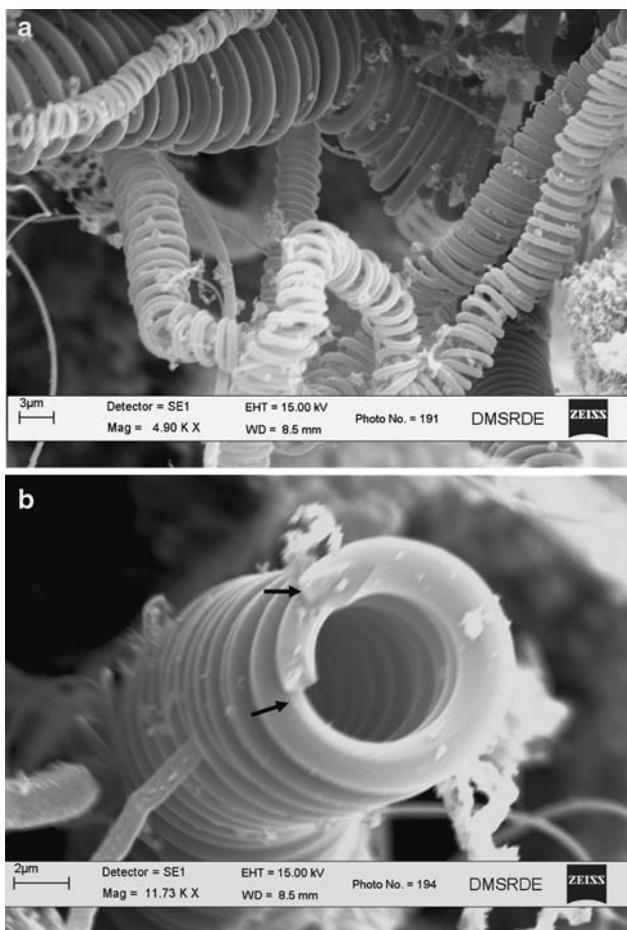
**Fig. 3** (a) Magnified view of bunch of double helical carbon microcoils present in the sample under SEM while (b) vertical projection through the channel of double helical carbon micro coils under SEM
