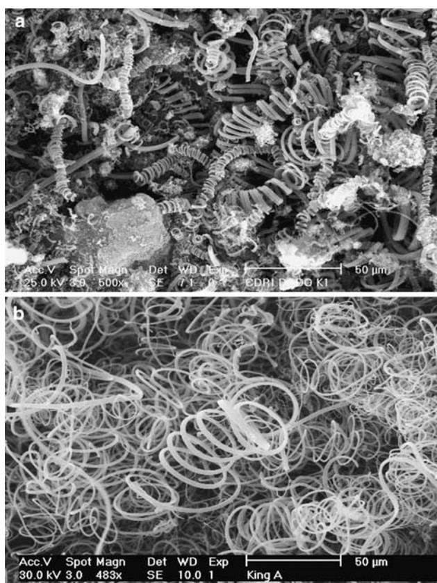
**Fig. 1** SEM images of carbon microcoils synthesized (a) in the presence of sulphur promoter (i.e., thiophene), (b) in the absence of a sulphur promoter
