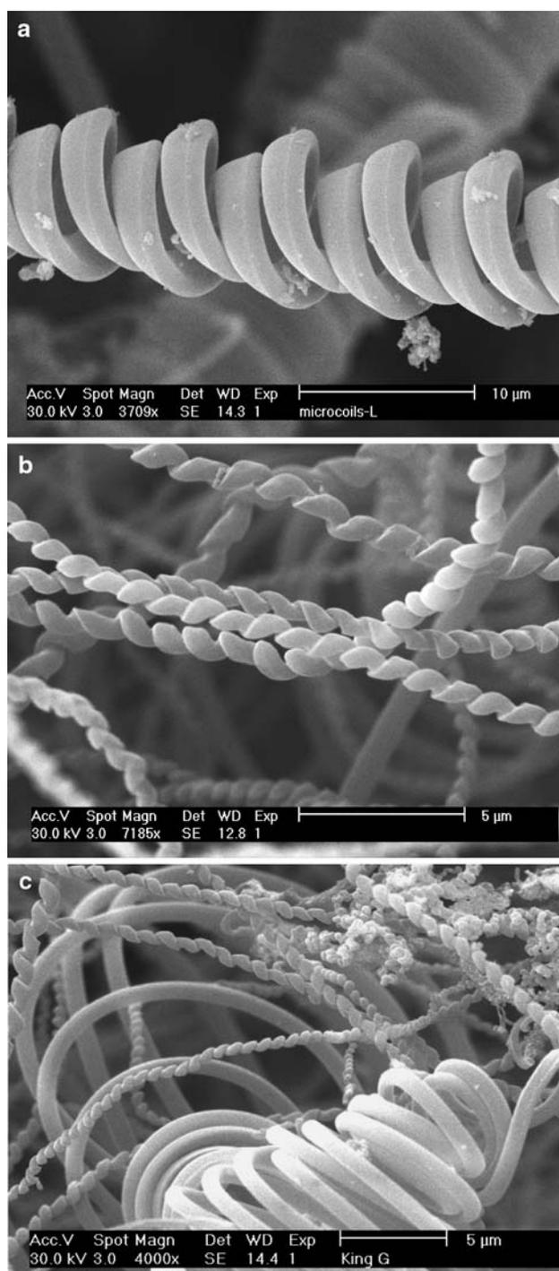
**Fig. 2** SEM images of (a) a typical double helical carbon microcoil, (b) a coiled carbon nanofiber synthesized under optimized conditions in the absence of thiophene, (c) part of sample containing both microcoils and coiled carbon nanofibers synthesized in the absence of thiophene
